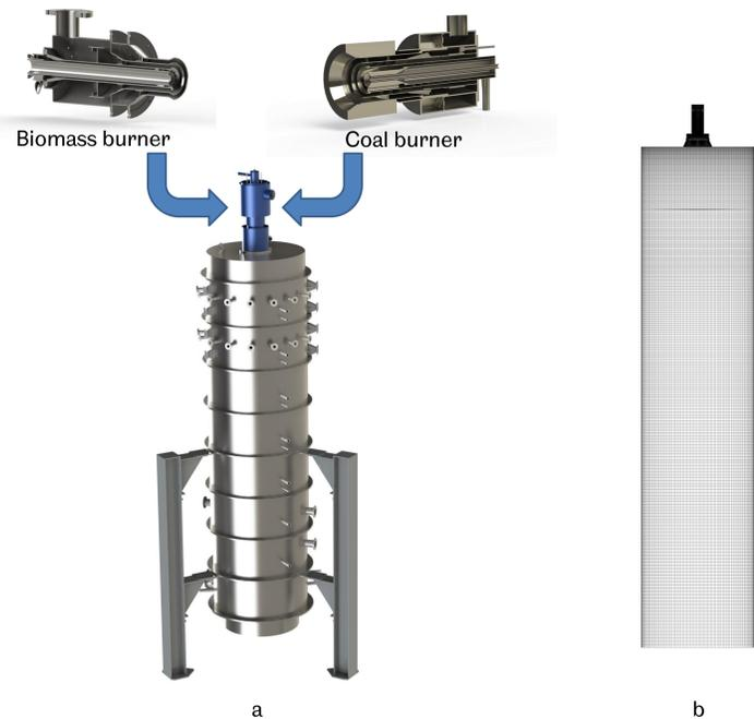
Figure 1. a) Computer representation of the UKCCSRC Pilot-scale Advanced Capture Technology (PACT) 250 kW combustion test rig. b) Computational domain used for LES computations consisting in 6.75 million hexahedral cells.
