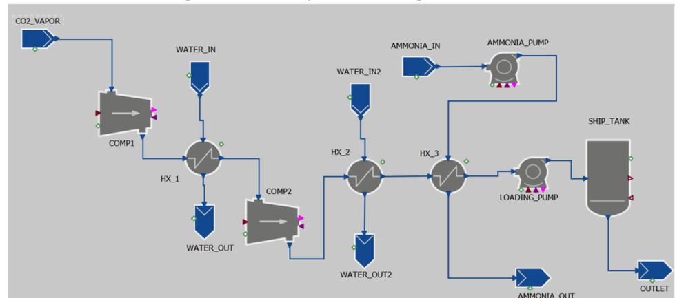
Figure 4: Multi-stage liquefaction and compression unit for the open cycle water/ammonia system for the ship transport of CO<sub>2</sub> to achieve the required condition
