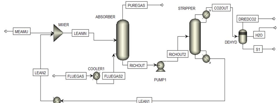
Figure 3: Carbon capture unit configuration unit
