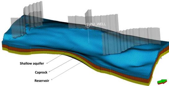
Fig. 1. The structural model of the numerical saline aquifer (36km x 10km) containing five major faults and three stratigraphic layers: reservoir layer, caprock (seal) layer and shallow aquifer layer.
