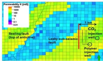
Fig. 2. Location of polymer injection well, sub-seismic fault and CO<sub>2</sub> injection well.
