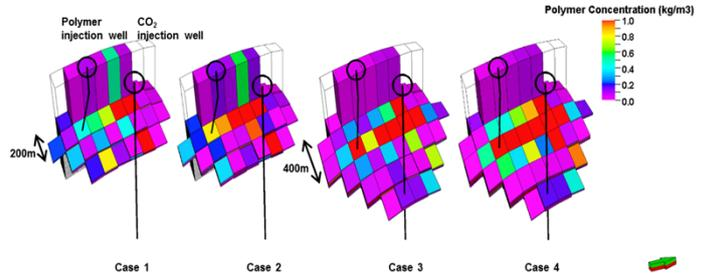
Fig. 4. The results of numerical simulations for polymer-gel injections at different distances to the leaky fault and with various viscosities.
