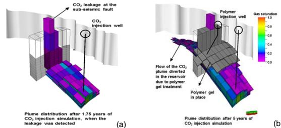
Fig. 5. The results of numerical simulations of CO<sub>2</sub> plume distribution: (a) at the time of leakage detection, and (b) after 5 years of post-remediation CO<sub>2</sub> injections.
