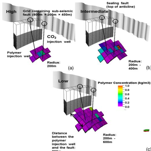
Fig. 3. Area of influence after 20 days of polymer-gel injections for a) high, b) intermediate, and c) low viscosity cases.
