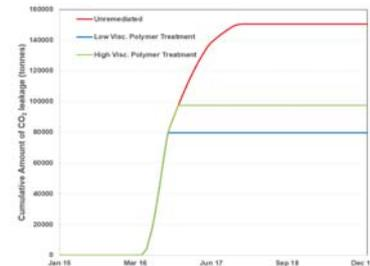
Fig. 6. The results of CO<sub>2</sub> leakage remediation for cases of un-remediated leakage, low and high viscosity polymer-gel treatments.
