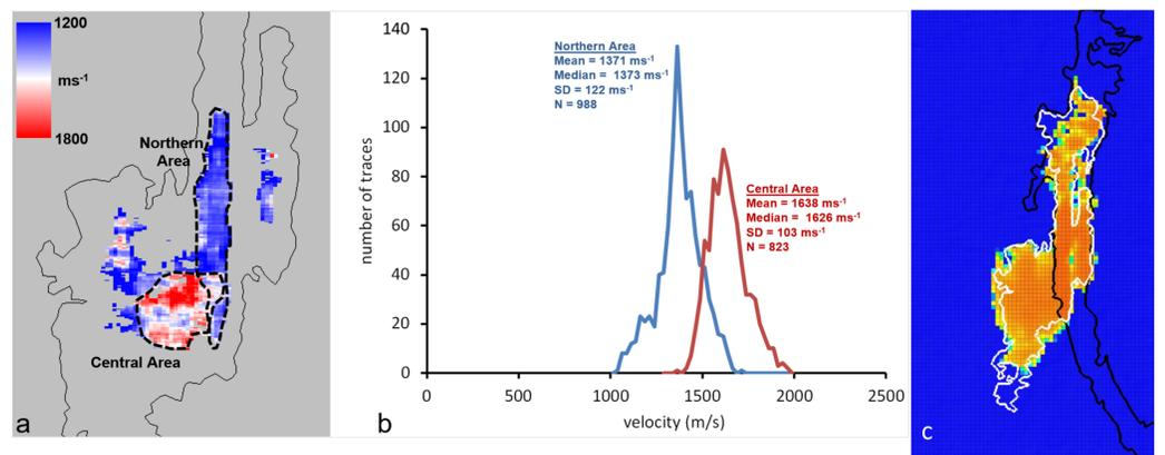
Fig. 2 Velocity analysis for two selected areas in the topmost CO<sub>2</sub> layer. a) Extracted velocities with areas marked. b) Velocity histograms for the two areas. c) Results of incorporating a high permeability channel into a reservoir model of the Sleipner site (white line shows CO<sub>2</sub>-water contact observed on seismic data; black line high permeability channel).
