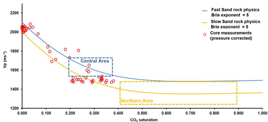
Fig. 1 Laboratory velocity-saturation measurements for Utsira Sandstone (Falcon-Suarez et al., 2018)
