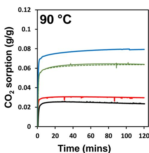
For all materials CO<sub>2</sub> uptake rate further increases at 90 °C, yet final capacity is reduced. 25:1 shows highest uptake at 0.079 g/g, while both 10:1 and 10:1 RBF have similar capacities. Uptake by 1:1 and 3:1 decreases by about 37% and reduces over time.
