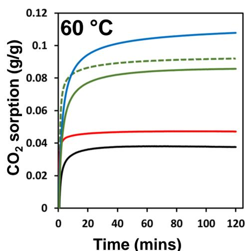
All materials sorb faster at 60 than 30 °C. 1:1 and 3:1 sorb about 25% less at 60 °C than 30 °C. 25:1 shows highest sorption with a final capacity of 0.108 g/g. 10:1 RBF reduces final capacity to 0.092 g/g, but 10:1 improves.
