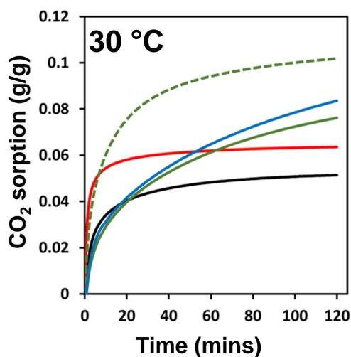
At 30 °C, 10:1 RBF shows highest sorption, reaching a final capacity of 0.102 g/g. Sorption is fastest for 1:1 and 3:1 but these have a lower uptake than 10:1 and 25:1, which show slower sorption.
