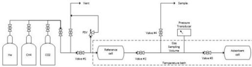
Manometric Adsorption Measurement Rig
