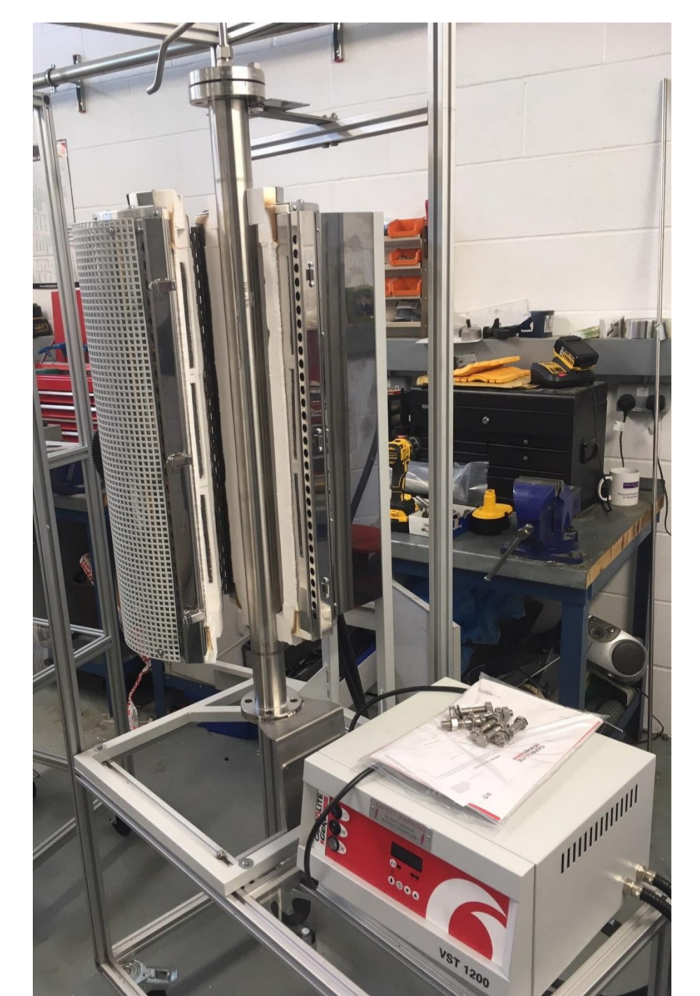
Reactor Material: stainless steel (253-MA) Temperature: up to 1000°C re: up to 10 bar (upgrade to 20 bar) Capacity: Up to 1 kg materials
