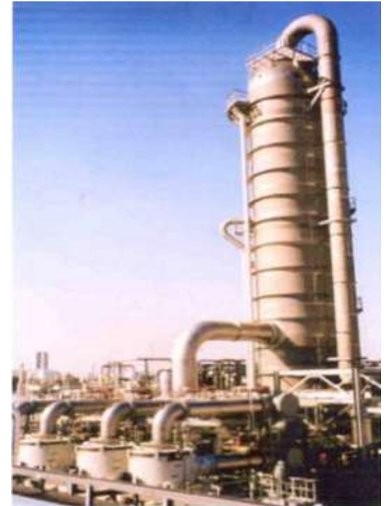
Rotating Packed Bed used for REACTIVE STRIPPING –40 times smaller plant (Dow Chemical, HOCl process)
